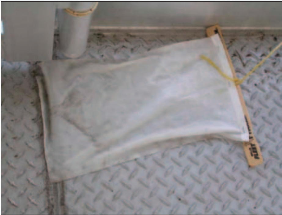
Figure 3: Method for calculating grams of residual moisture collected in a drag swab that had been weighed dry, dragged over the floor surface of a pig transport trailer (Figure 2), then placed in the bucket of a kitchen scale and weighed again.
