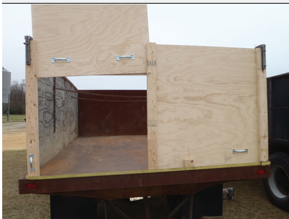
Figure 1: A standard dump trailer or truck modified for use as a swine euthanasia chamber. A sliding tailgate section and top hinges added to this truck bed facilitates loading of live pigs and then dumping the carcasses once the pigs have been euthanized. The sides and tailgate are sealed with expanding foam to form a gas-tight seal. A tarpaulin or plastic sheeting is placed over the truck bed to reduce air mixing and carbon dioxide washout.
