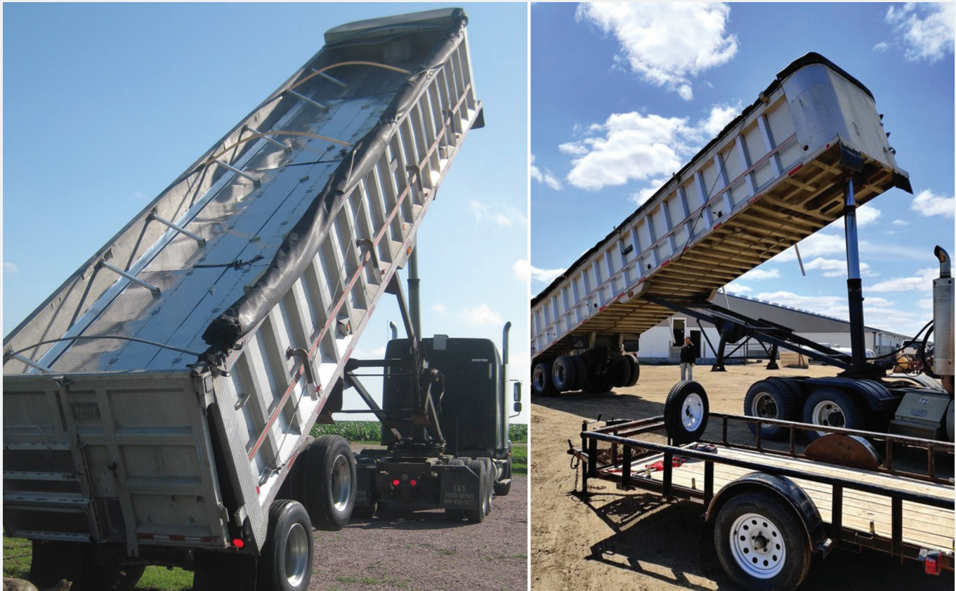
Figure 6: Hydraulic dump trailer in a raised position for easy emptying of carcasses. The trailer can be moved to place carcasses in a designated location.
