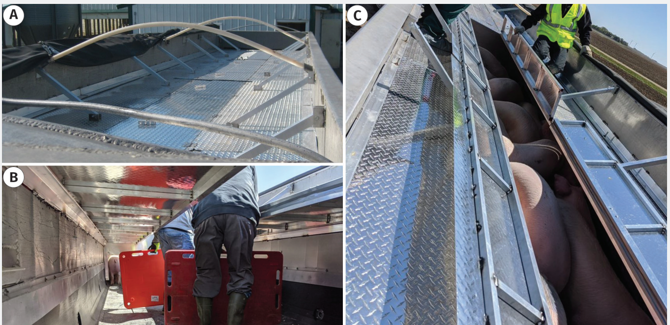
Figure 2: Installed ceiling in the trailer with hinged center. A) The ceiling decreased the area needed to be filled with CO 2 and prevented pigs from raising their heads above the gas. B) The hinged center provided a space for people to walk while loading pigs onto the trailer that could be closed later. C) The overlapping lip on one side of the lifttable hinged panels prevented the formation of a gap.
