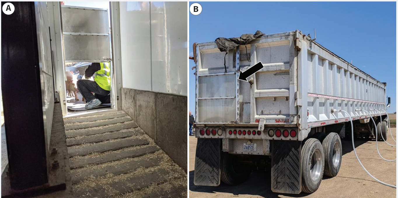
Figure 1: Rear of the trailer with a vertical sliding door installed for loading pigs. A) The vertical sliding door open and trailer backed up to barn chute for loading pigs. B) The trailer with the closed vertical sliding door (arrow).
