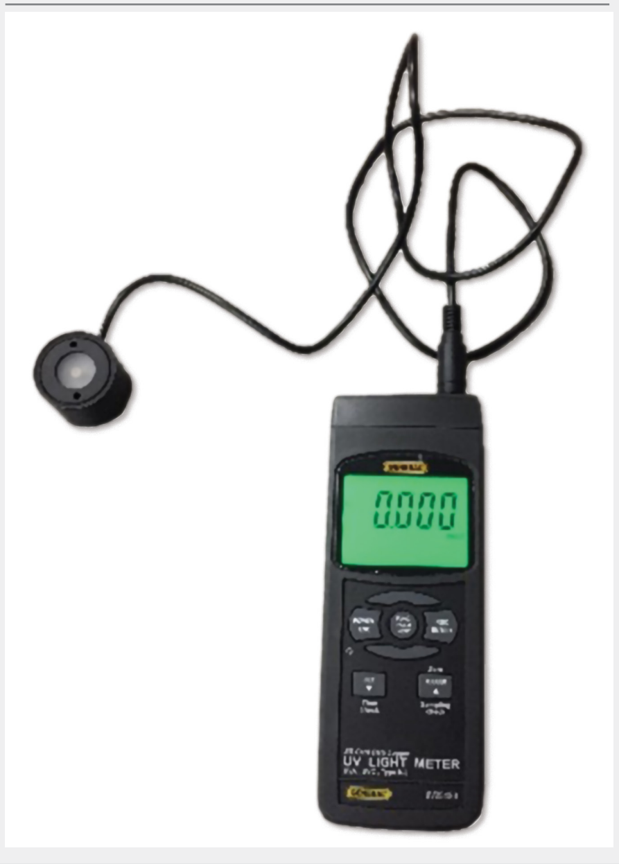
Figure 1: A portable, simple UV light meter (UV512C Digital UVC meter, General Tools & Instruments LLC) with a plugged-in sensor that can measure either UVC or UVA, with a data-logging SD card.
